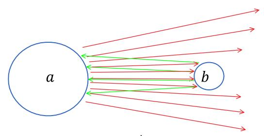
In the figure above, the circles labeled a and b respectively represent two different types of particles electromagnetically interacting. The red and green arrows indicate the direction of polarizations of the preonic field from a and b. The momentum that can be imparted to one particle interacting by the other's polarized field is  $\Delta \vec{P}_a \propto \frac{\left\|\vec{\Theta}_b^{+/-}\right\| \left\|\vec{S}_a\right\|}{r^2}$  (green arrows) and
